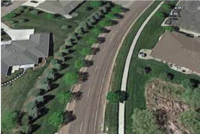
Ralph Rogers Ave in Sioux Falls, South Dakota. An example of a multi-use shoulder that accommodates but is not restricted to bicycle travel
