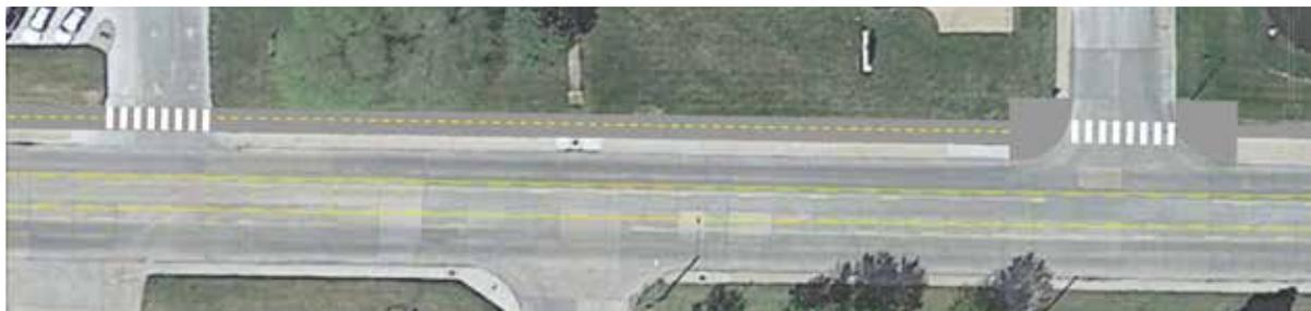
Faidley sidepath concept. In this segment, new sidepath is located adjacent to the existing back of curb sidewalk, using the existing facility as a buffer from the travel lanes. High visibility crosswalks are used to mark street and major driveway interruptions.
