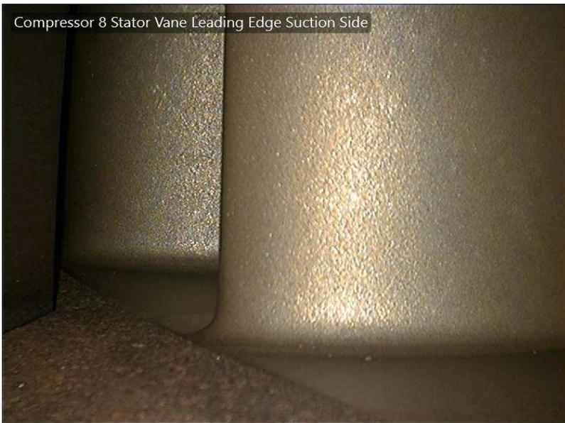
Compressor 8 Stator Vane Leading Edge Suction Side
