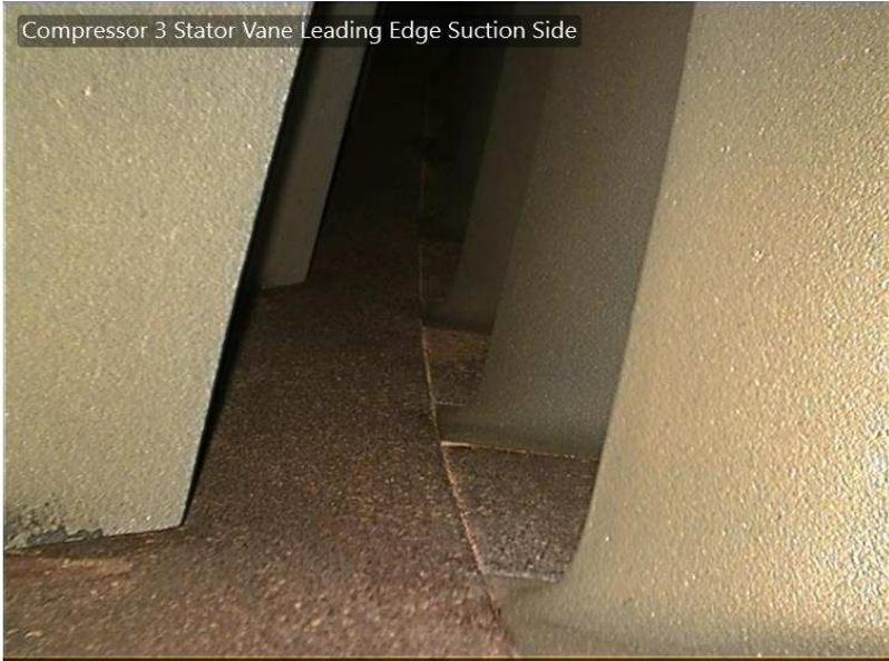
Compressor 3 Stator Vane Leading Edge Suction Side
