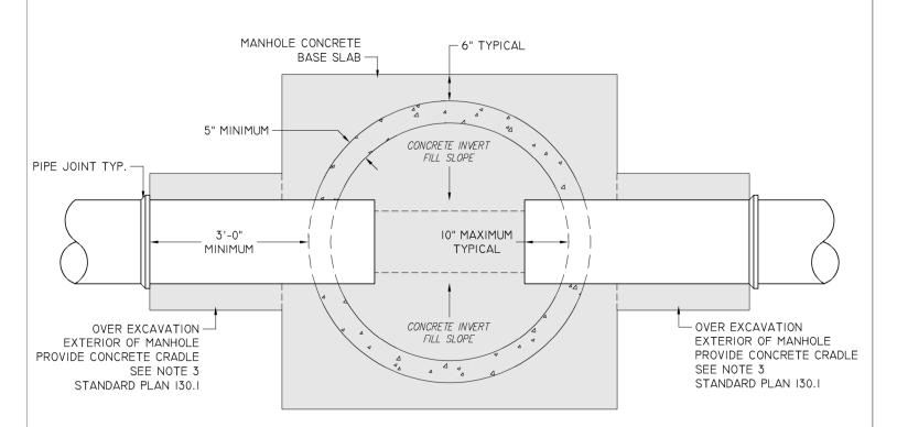
SANITARY SEWER MANHOLE BASE PLAN VIEW
