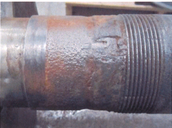
Pump shaft corrosion
