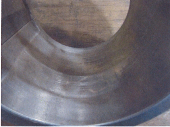
Typical light bearing wear
