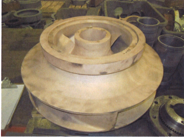
Impeller with TE case ring installed
