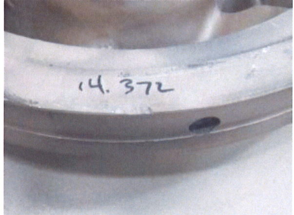
Impeller CE with case ring OD wear (step)
